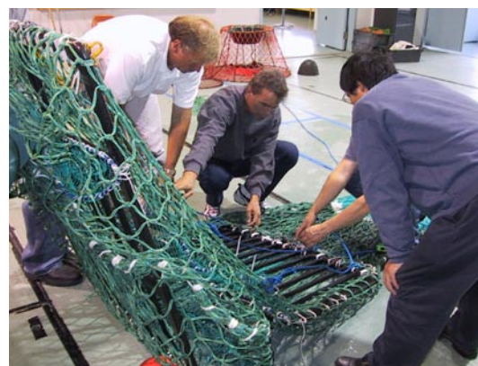
Pingguo He, right, back to camera, works with fishermen from Poland, Maine, on a fishing net designed to catch flat fish, but let cod escape.
