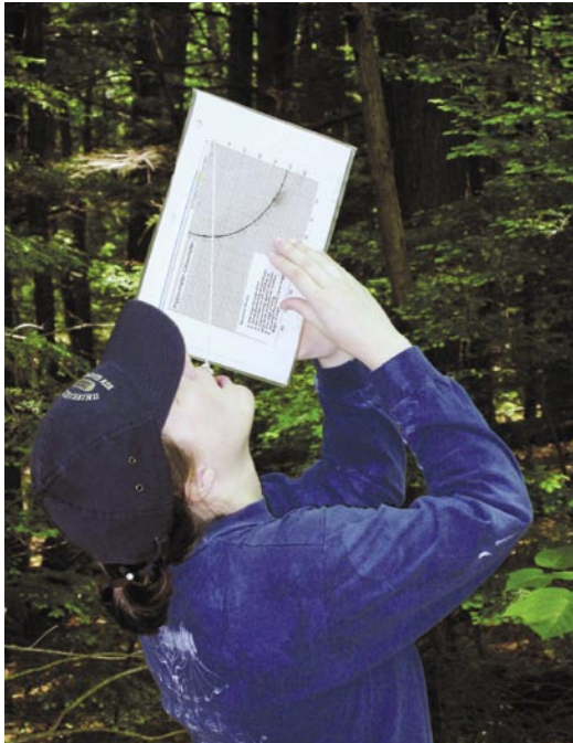
A student uses a rudimentary clinometer to measure tree height, which can be used to determine the biomass of a forest and, in turn, can be an indicator of forest health.
