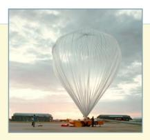
A balloon like this, thinner than a garbage bag and filled with six million cubic feet of helium, will haul the 2.5 ton BalloonWinds payload aloft to 100,000 ft. Photo courtesy of Holloman Air Force Base
