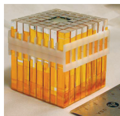
This array of gamma-ray sensitive material, called “scintillators,” make up a single GRAPE detector.
