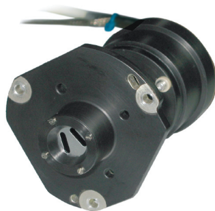
The IBEX star sensor showing the V-shaped aperture. Photos: David Heitzler, UNH-SSC
