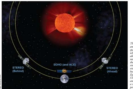
The SOHO and ACE spacecraft, which orbit about 1 million miles closer to the Sun, provide a head-on view of what's headed toward Earth while STEREO A and B allow a side view perspective.
